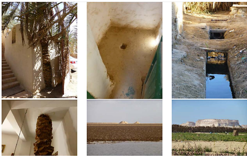
Figure 11: Respect to nature represented in integration of Palms within structures to avoid cutting them (left); sensible use of water in dry toilet (top-middle) and reuse of sewage water (top-right); use of Kourshif as natural building material (bottom-middle) and finally avoid building and development in agricultural areas (bottom-right) (Source: the author – various trips).
