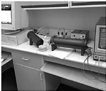
Figure 1: Schematic diagram of apparatus for measuring sound absorption coefficient.
