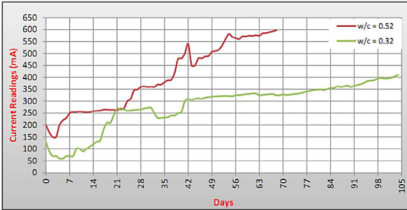
Figure 7: Current readings for un-coated deformed steel bars in 44MPa concrete cylinders.
