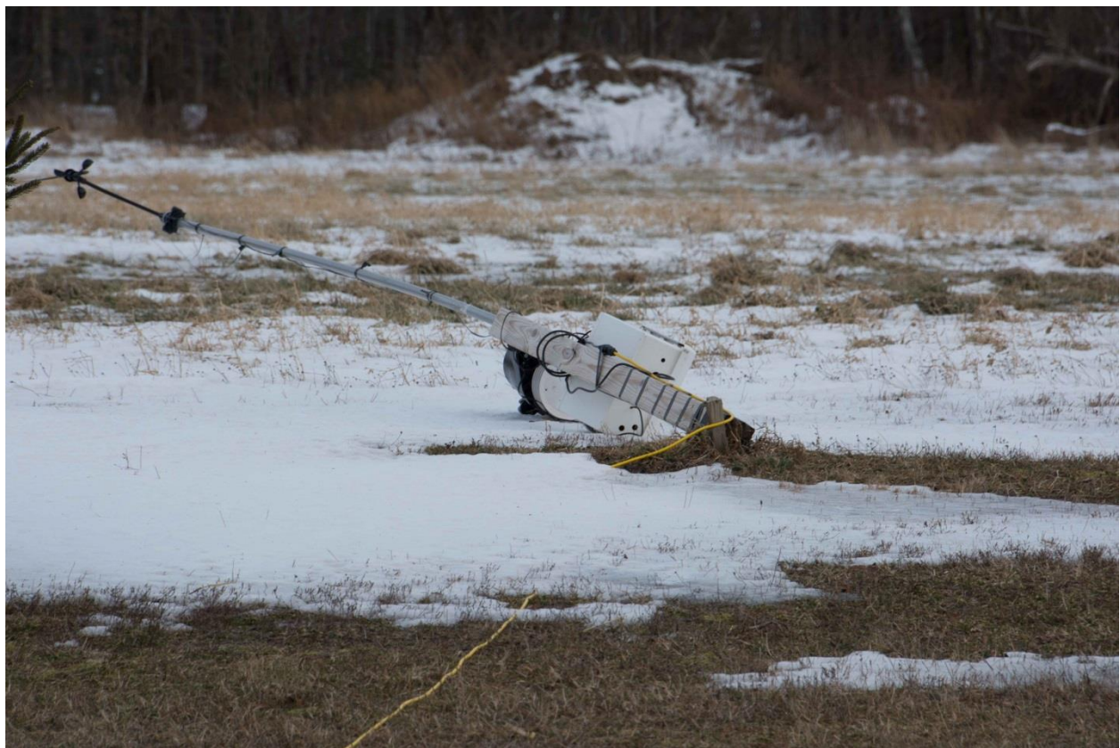
Figure 1: Climate Station at Glen Valley blown down by wind gust on January 5, 2018
