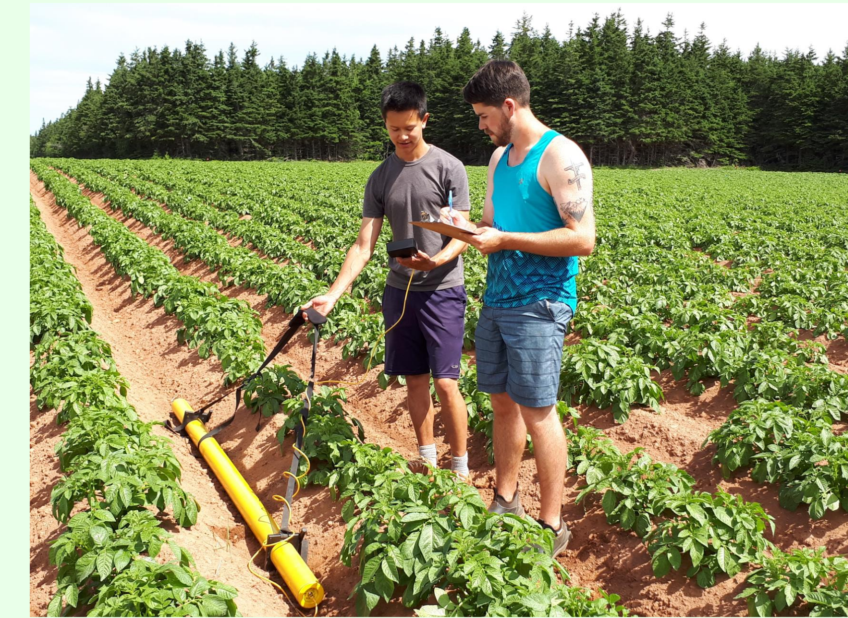
Fig. 3 Data collection of HCP using the Dual EM-2
