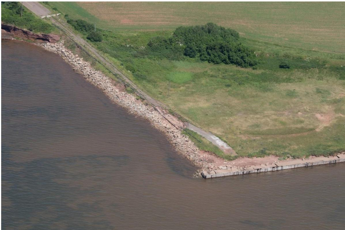
Figure 1 –Brae Harbour Road and Wharf Abandoned due to Coastal Erosion
